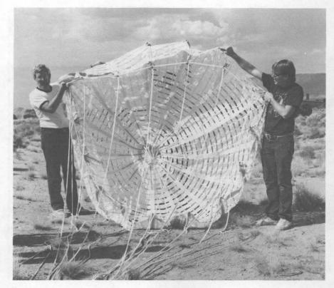
DISPLAYING AN 11.6-footdiameter pilot chute like the one used by NASA in its solid-fuel rocket booster chute system are Bruce Rutledge (left) and Fred Hillebrandt (both contractors). The pilot chute creates the force necessary to deploy a larger drogue shoot, which stabilizes and directs the boosters. Both participated in the recent chute test along with Sandia scientists and NASA representatives.
